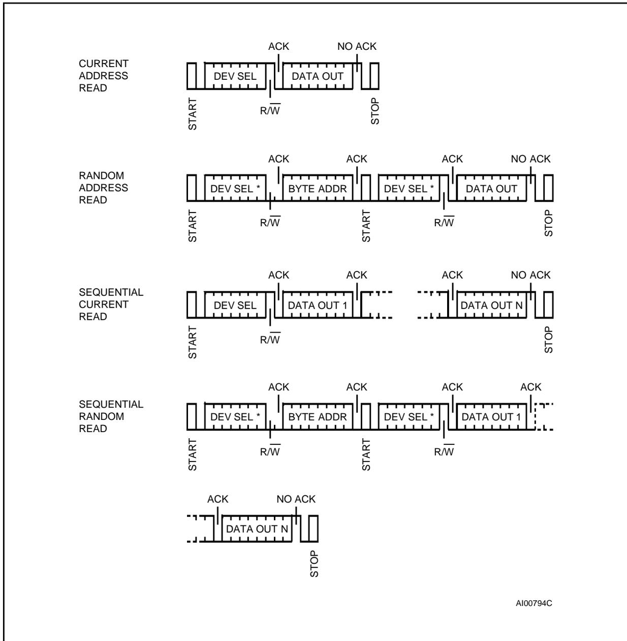
Note: \* The 7 Most Significant bits of DEV SEL bytes of a Random Read (1st byte and 3rd byte) must be identical.
