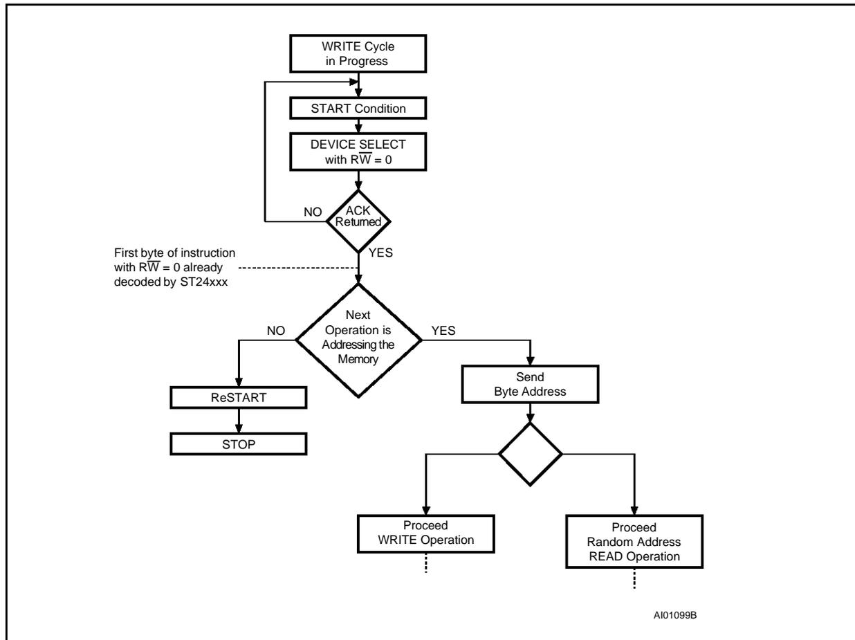
Figure 9. Write Modes Sequence (ST24/25C04 and ST24C04R)
